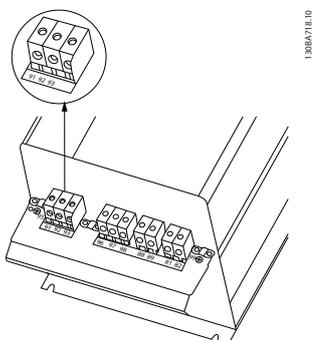
Illustration 6.12 Mains Connection Enclosure Type C3 (IP20).
