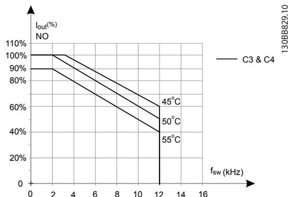
Illustration 9.17 Derating of I<sub>out</sub> for different T<sub>AMB, MAX</sub> for enclosure types C3 and C4, using 60° AVM in Normal overload mode (110% over torque)
