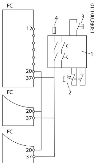
Illustration 2.6 Paralleling of Multiple Frequency Converters Example
