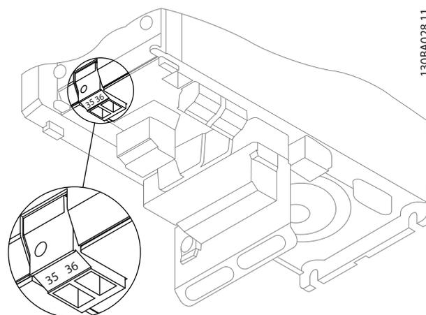
Illustration 3.10 Connection to 24 V Back-up Supplier (A2-A3).
