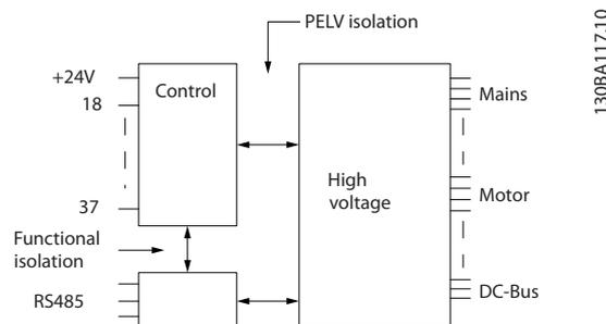
Illustration 9.1 PELV Isolation of Analog Inputs
