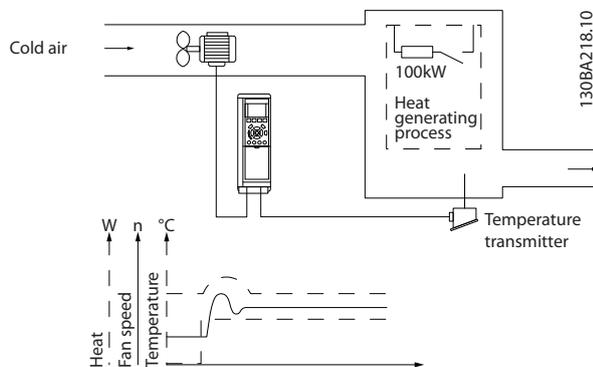
Illustration 2.30 Closed Loop Control for a Ventilation System
