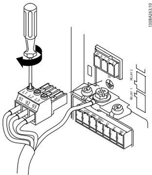
Illustration 6.4 Mounting Mains Plug and Tightening Wires
