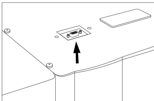
Illustration 6.46 Top Connection for Fieldbus on IP00
