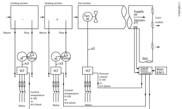
Illustration 2.16 Fan System Controlled by Frequency Converters.
