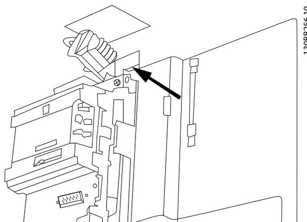
Illustration 6.47 Top Connection for Fieldbus NEMA 1 Units
