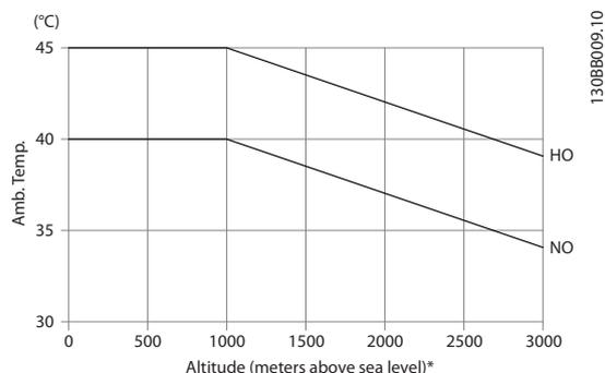
**Illustration 9.26** Example: At an altitude of 2000 m and a temperature of 45 ° C (T<sub>AMB, MAX</sub> - 3.3 K), 91% of the rated output current is available. At a temperature of 41.7 ° C, 100% of the rated output current is available
