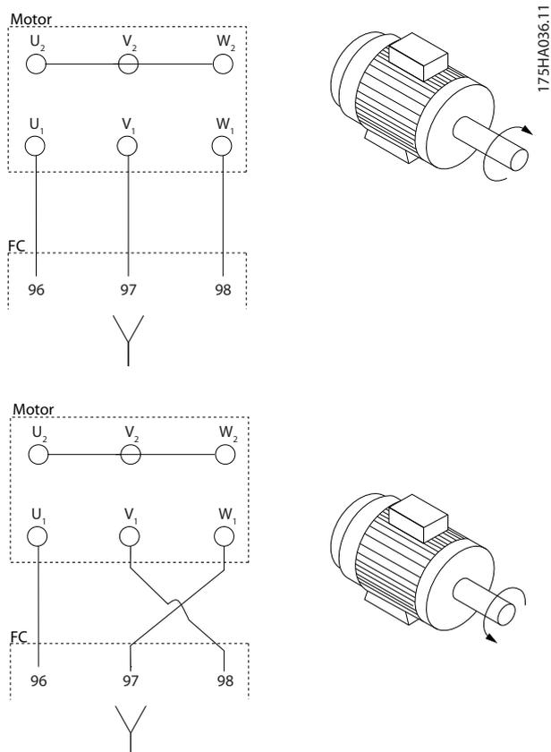
Illustration 6.40 Terminal Connection for Clockwise and Counter-clockwise Rotation
