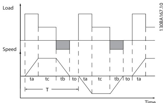
Illustration 2.39 Intermittent Duty Cycle for the Resistor
