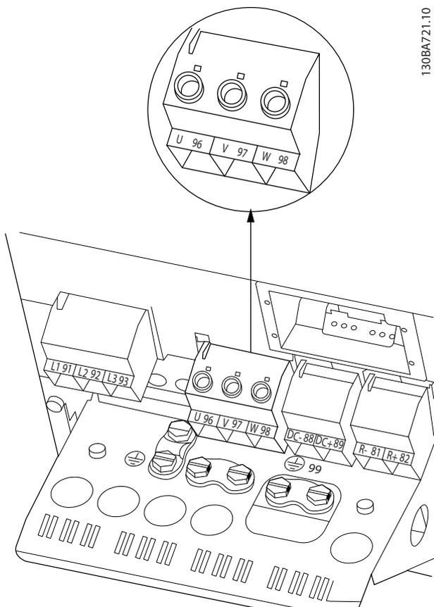
Illustration 6.17 Motor Connection for Enclosure Type B4
