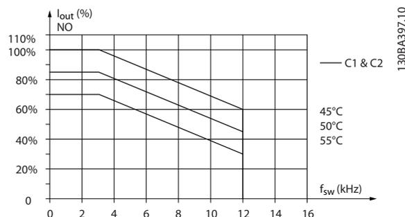
Illustration 9.16 Derating of I<sub>out</sub> for different T<sub>AMB, MAX</sub> for enclosure types C1 and C2, using 60° AVM in Normal overload mode (110% over torque)
