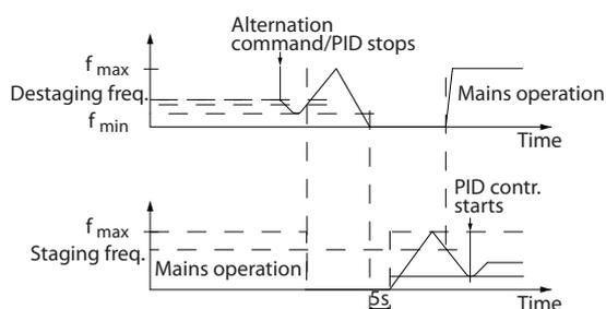
Illustration 7.8 Pump Staging with Lead Pump Alternation
