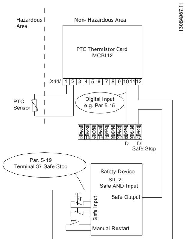
**Illustration 2.7** Illustration of the essential aspects for installing a combination of a Safe Torque Off application and a MCB 112 application. The diagram shows a Restart input for the external Safety Device. This means that in this installation 5-19 Terminal 37 Safe Stop might be set to value [7] PTC 1 & Relay W or [8] [8] PTC 1 & Relay A/W. Refer to MCB 112 operating instructions for further details.
