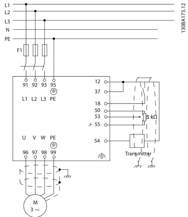
Illustration 2.31 Example of Closed Loop PID Control
