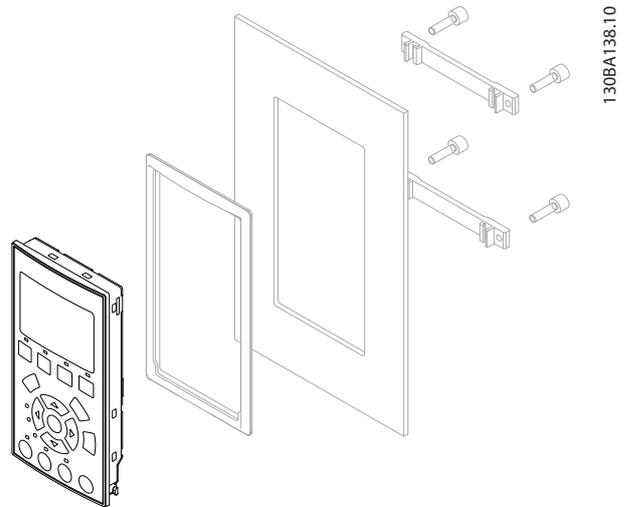
Illustration 3.16 LCP Kit with Graphical LCP, Fasteners, 3 m Cable and Gasket
