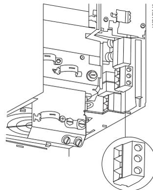
Illustration 6.9 Mains Connection Enclosure Type B3 (IP20)
