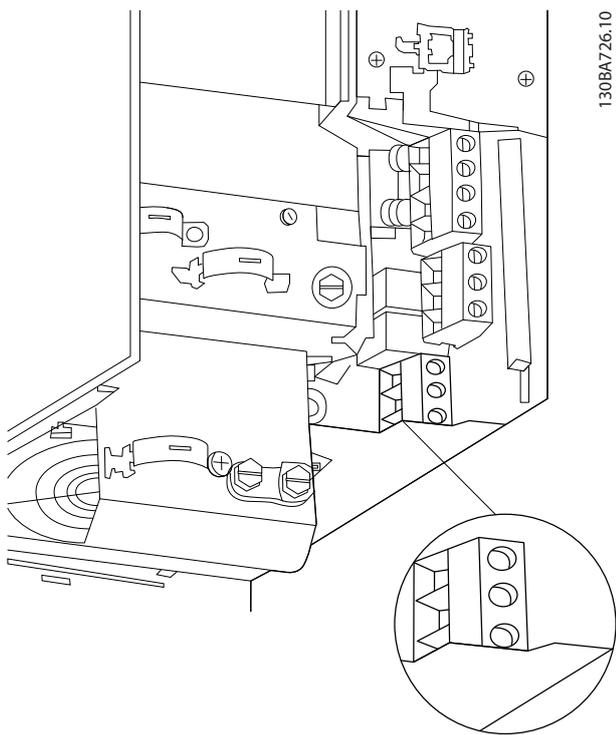
Illustration 6.16 Motor Connection for Enclosure Type B3
