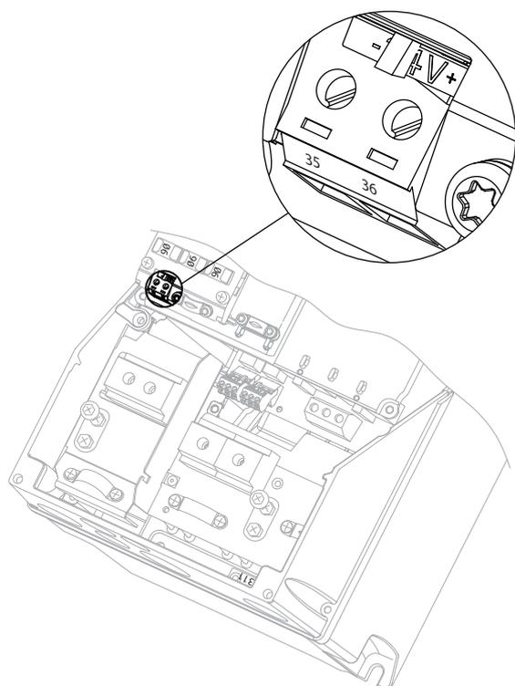
Illustration 3.11 Connection to 24 V Back-up Supplier (A5-C2).
