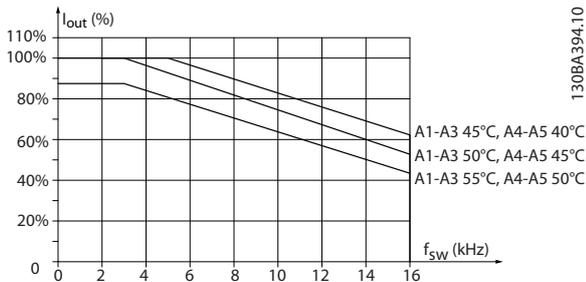
Illustration 9.5 Derating of  $I_{out}$  for Different  $T_{AMB, MAX}$  for Enclosures Type A, using 60° AVM and maximum 10 m motor cable
