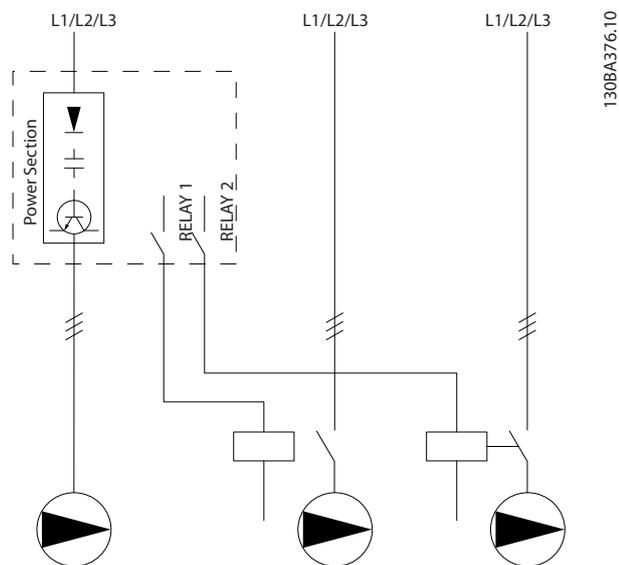
Illustration 7.9 Fixed Variable Speed Pump Wiring Diagram
