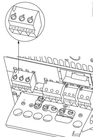
Illustration 6.10 Mains Connection Enclosure Type B4 (IP20)
