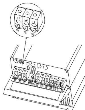
Illustration 6.13 Mains Connection Enclosure Type C4 (IP20).
