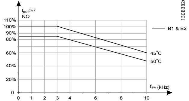
Illustration 9.12 Output current derating with switching frequency and ambient temperature for 600 V frequency converters, enclosure type B, 60 AVM, NO
