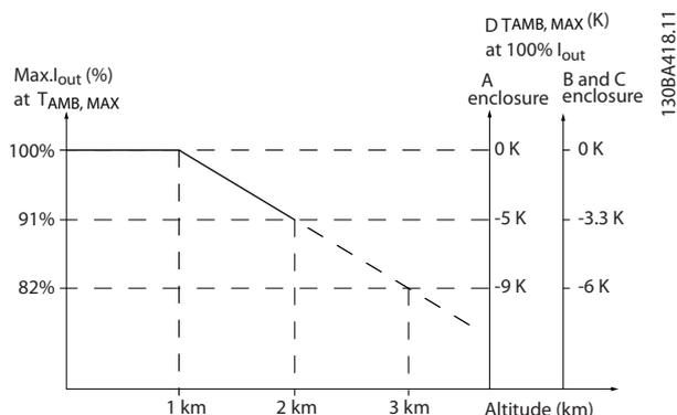
**Illustration 9.24** Derating of output current versus altitude at T<sub>AMB, MAX</sub> for enclosure types A, B and C. At altitudes above 2000 m, contact Danfoss regarding PELV.
