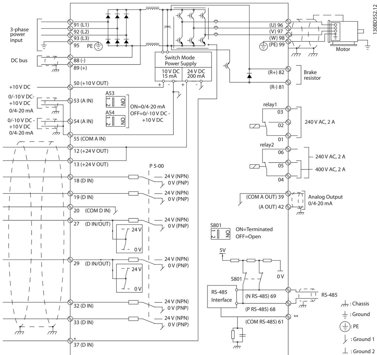
Illustration 6.55 Basic Wiring Schematic
