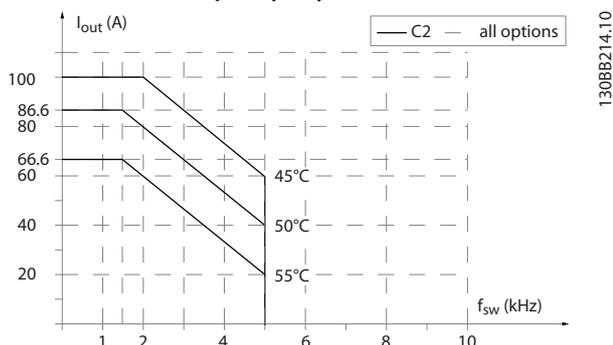
**Illustration 9.23** Output current derating with switching frequency and ambient temperature for enclosure type C2, SFAVM. Note: The graph is drawn with the current as absolute value and is valid for both high and normal overload.
