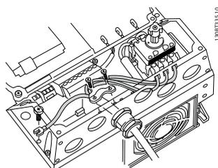
Illustration 6.7 Connecting to Mains and Earthing with Disconnecter
