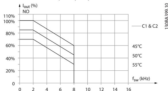
Illustration 9.18 Derating of I<sub>out</sub> for different T<sub>AMB, MAX</sub> for enclosure types C1 and C2, using SFAVM in Normal overload mode (110% over torque)
