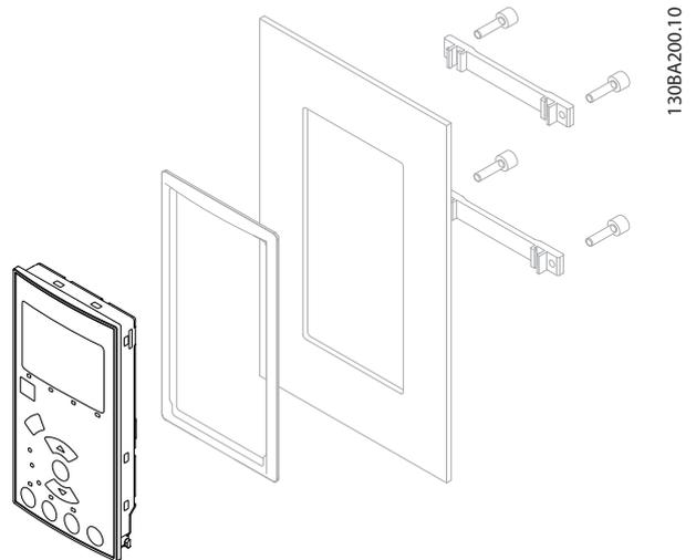
Illustration 3.17 LCP Kit with Numerical LCP, Fasteners and Gasket
